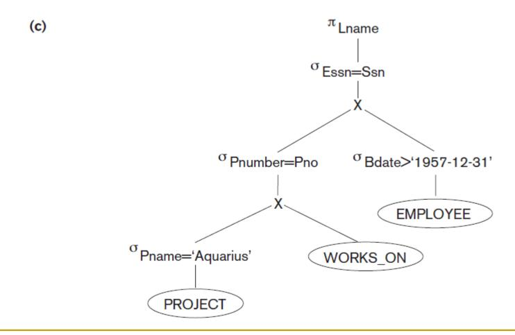
**Step 4:** Replacing Cartesian Product and Select with Join operation.
