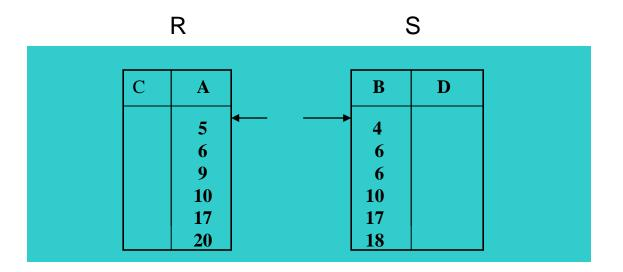
Assume that A is a key of R. Initially, two pointers are used to point to the two tuples of the two relations that have the smallest values of the two joining attributes.
